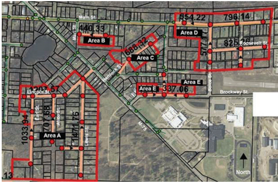
Green Dots and Lines are existing sanitary sewer manholes and mains Red dots and pink streets show proposed new sanitary sewer manholes and areas to be served.
